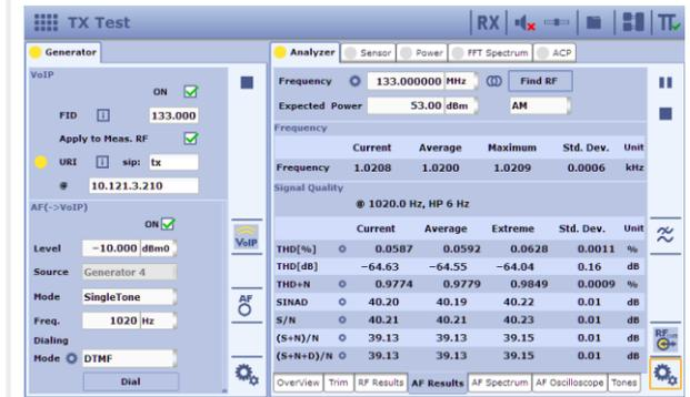
Integrated VOIP generator for testing air traffic controller equipment in accordance with ED-137B.
