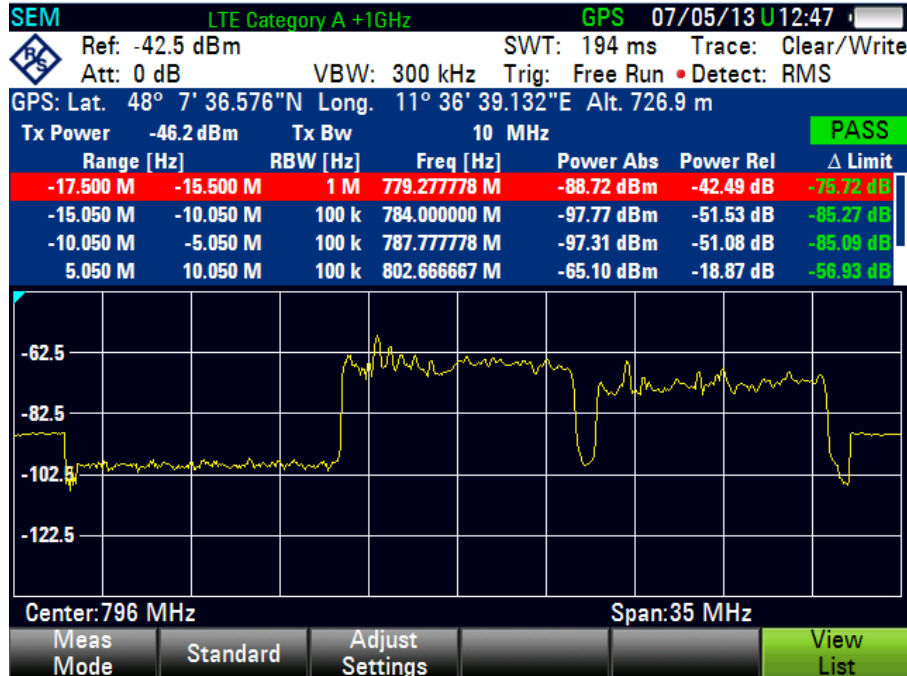
Fig. 25 SEM OTA measurement of a 10 MHz FDD LTE signal.
