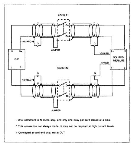
Figure 2-6. Source with External Sense or Kelvin Measurement
