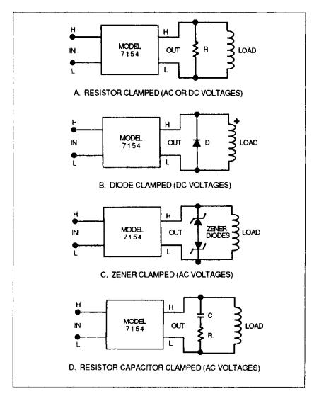
Figure 2-2. Limiting Inductive Reaction Voltage
