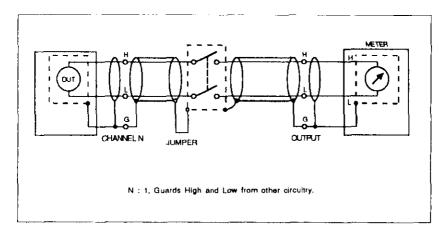
Figure 2-4. Guarded Floating Measurement
