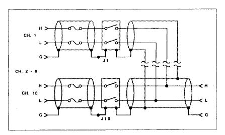
Figure 1-1. Model 7154 Simplified Schematic
