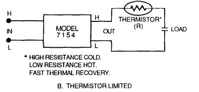
Figure 2-1. Limiting Capacitive Reaction Current
