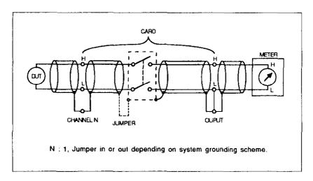
Figure 2-3. Shielded Floating Measurement
