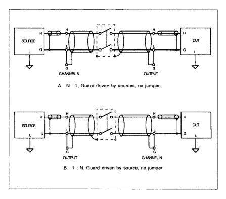
Figure 2-5. Single-Pole Switch with Switched Guard
