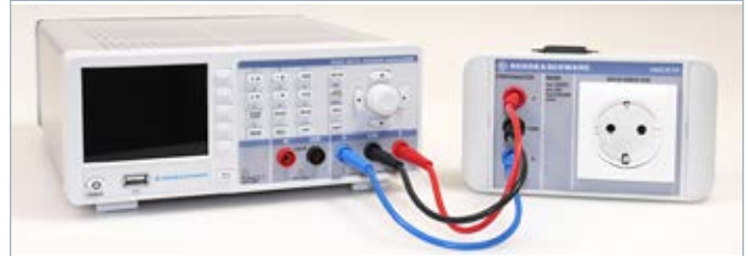
Fig. 4.1: Connecting HZC815 DE version to R&amp;S®HMC8015.
