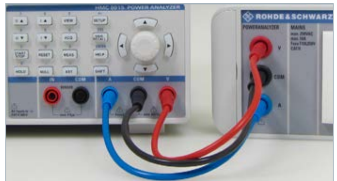
Fig. 4.6: Voltage-based measurement, wiring example.
