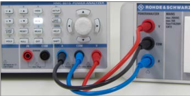
Fig. 4.8: Current-based measurement, wiring example.
