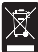
Fig. 1.4: Product labeling in accordance with EN 50419
