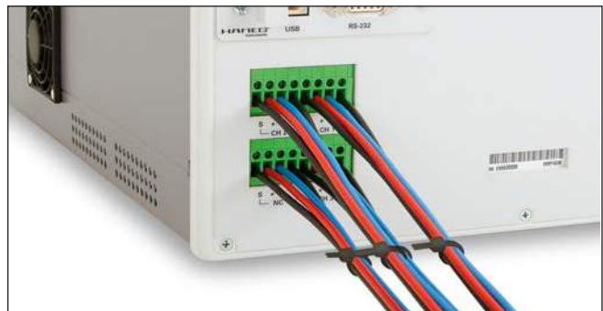
Fig. 3.4: R&S®HMP4040 terminal strip on the back panel of the instrument
