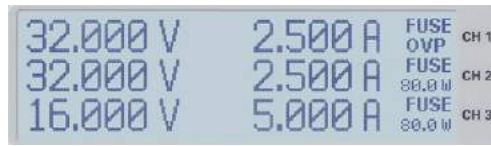
Abb. 5.4: Over Voltage Protection (R&S®HMP2030)
