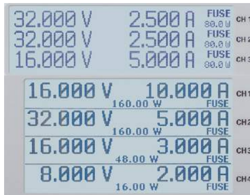
Fig. 4.7: R&S®HMP2030/ R&S®HMP4040 Fuse appearance in the display
