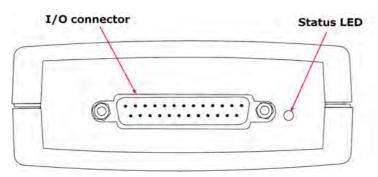
**I/O connector:** for the pin-numbering of the I/O connector, see <u>I/O connector pins</u>. The Pico PP545 Small Terminal Board is specially designed to connect to this socket to allow you to make connections to individual wires easily without soldering. If you need to use a ribbon cable to connect your signals to this socket, use the shortest possible length to avoid introducing too much crosstalk between the signals.
